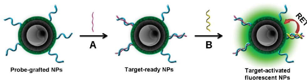
Figure 1. Principle of DNA detection on fluorescent multilayer core–shell NPs: (a) target-ready NPs are prepared by complexing ssDNA probe-grafted NPs with polymer transducer; (b) hybridization of target DNA with ssDNA probes activates the polymer transducer as energy donor toward dye-doped silica shell and excitation at 410 nm generates fluorescence emission by acceptor molecules at 550 nm.
